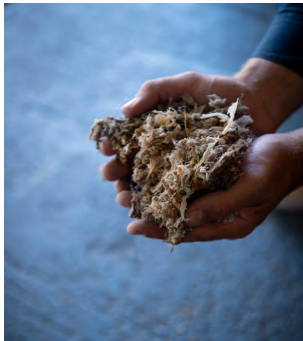
ABOVE: Refuse Derived Fuel, used at Adelaide Brighton Cement's Birkenhead manufacturing facility
